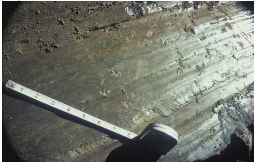
Fig 3.7.14 Basal shear surface with striations and polish in clay-rich head deposits, Sevenoaks, Kent, England. Scale in inches. (J.N. Hutchinson)
